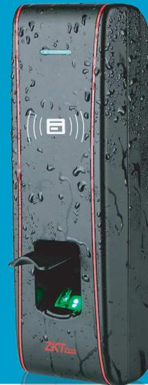
F16 is a fingerprint access control terminal with an integrated proximity reader (EM). It is IP65 rated which enables it to be resistant from water, dust and other outside damages. It can be installed easily on your network having both Ethernet and RS485 serial ports. Weigand-OUT port allows connection of reader to ZK or any 3rd party access control panels panel. Using Weigand-In port, you can connect to any card readers for authentication at both entrance and exit.
